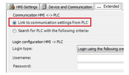
Simplified communication settings in CODESYS HMI: Use of current communication settings (device name, IP address)
