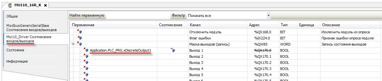
The screenshot shows the configuration interface for the MU110\_16R\_K template. The sidebar and table structure are similar. The highlighted row for Application.PLC\_PRG.xDiscreteOutput1 is assigned to 'Выход 1' (Output 1) with address %QX170.0, type BOOL, unit Запись состояния выходов (Recording of output status), and description Выход 1 (Output 1). Other outputs from 2 to 6 are listed below.
