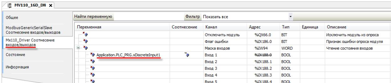
The screenshot shows the configuration interface for the MV110\_16D\_DN template. The sidebar and table structure are similar to the previous one. The highlighted row for Application.PLC\_PRG.xDiscreteInput1 is assigned to 'Вход 1' (Input 1) with address %IX188.0, type BOOL, unit Чтение состояния входов (Reading of input status), and description Вход 1 (Input 1). Other inputs from 2 to 5 are listed below.
